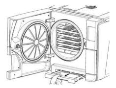
3 Lift the used filter from the handle and remove it.
