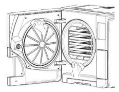
5 Insert the new seal and press first up and down.
