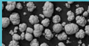
KaVo's PROPHYpearls without corners or edges. (Grain size 60–70 µm).
