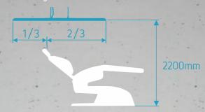
The height of the luminaire should be about 800-1200 mm above the working area.
