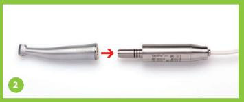
Connect the contra-angle (ISO E-connection) with the motor (must not be rotated).
