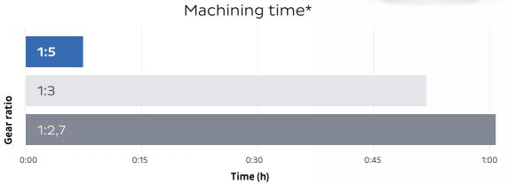
$<sup>^{\</sup>star}$  Representation of the average period of time for cutting through a defined sample of zirconium oxide
