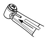
▶ Carefully plug the coolant hose in central position onto the media tube proceeding in axial direction.
