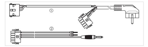
Using the measuring cable ① the unit is disconnected from the mains supply and connection of the treatment centre to the sight window is enabled. Hence, the customer-provided mains supply L & N on the power input board need not be disconnected. The adapter cable ② is included in the delivery of the KaVo measuring cable and is required for older treatment centres that are not equipped with an X2 connector.
