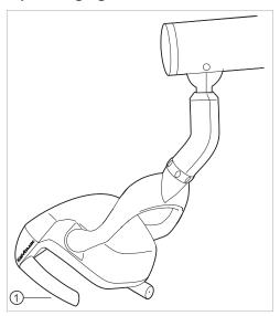
Fastening screw of the handle support when the gripping sleeve has been removed
