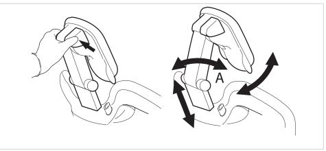
► Press the lock button and swing the headrest into the desired position.
