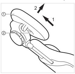
► To remove the headrest cushion, remove the screw ②, pull the cushion ① up slightly, and remove it to the front.
