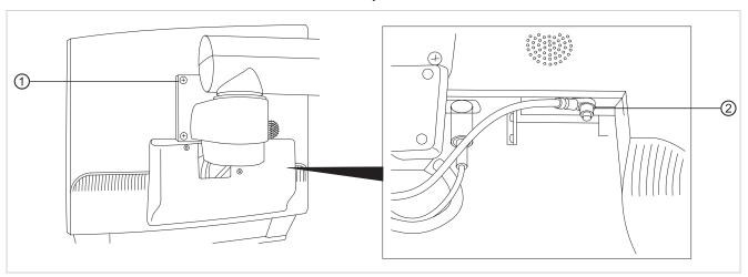
► Touch measuring point ① with the test tip.
