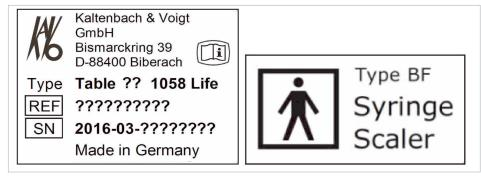
Nameplate dentist element (e.g. table TM) / marking of the applied parts of type BF
