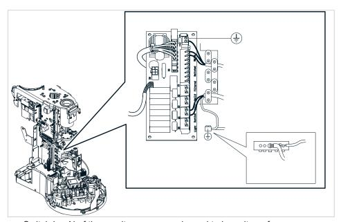
► Switch L + N of the on-site power supply cord to be voltage-free.
