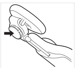
► To swing the headrest, turn the locking dial to the left, move the headrest into position, and turn the dial to the right to lock it.
