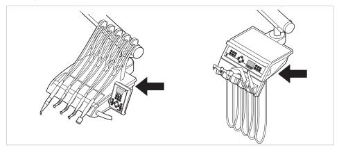
Site of attachment of rating plate and type BF applied parts ID on dentist element
