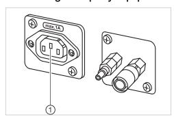
▶ Position the test tip on the middle contact ①.
